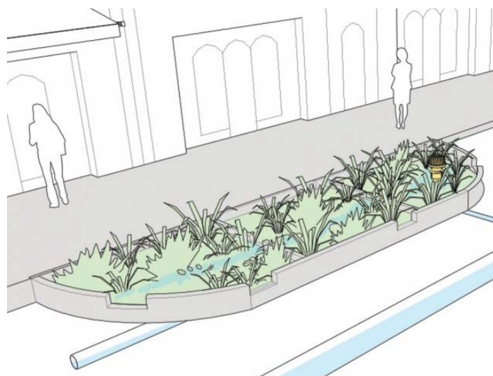
Figure 4 – Typical On-Street Bioswale Application Source: National Association of City Transportation Officials (NACTO)
